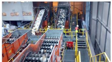
Figure 4: Bywaters MRF paper and cardboard sorting machinery
